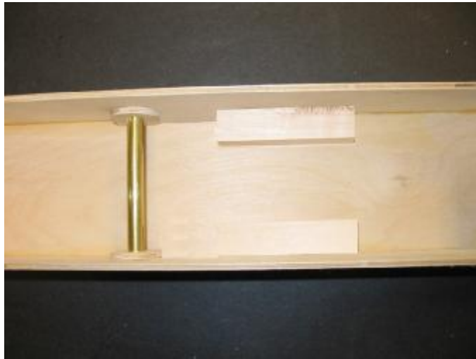
Engine rails glued in 3 inches in front of bulkhead 2.
