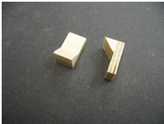
Throttle servo rails ready to glue to tub.
