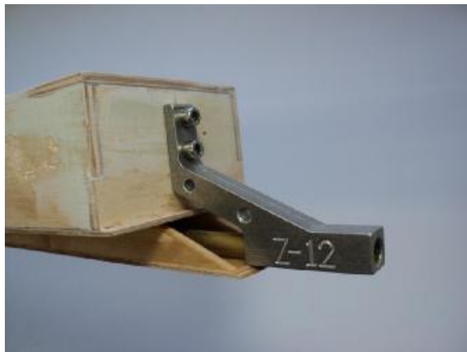
Strut in place on ski. 12G kit shown. 21 the same.
