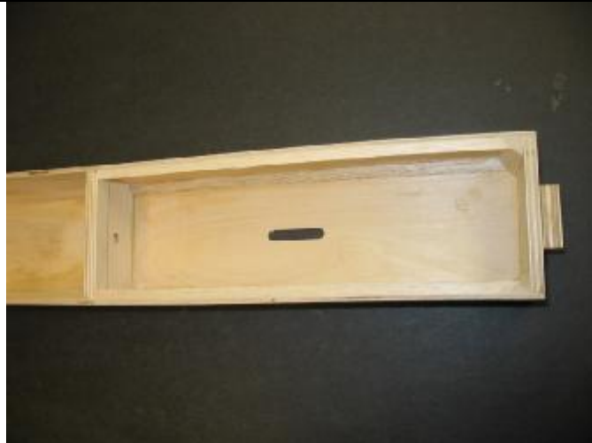
Upper tri stock in place. Note 5/16 tri on transom.
