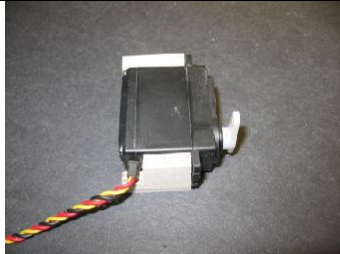
Side trimmed for servo wire clearance,
