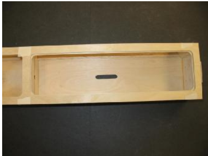
Tub top in place. Note that it is centered on radio box lip.
