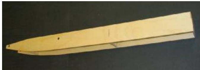
Tub sides glued to bulkheads.
