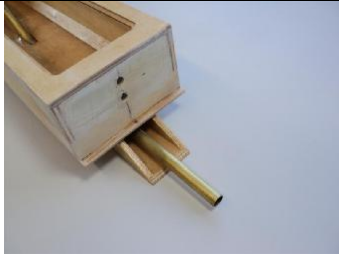
Be sure to leave enough shaft tube for the strut.
