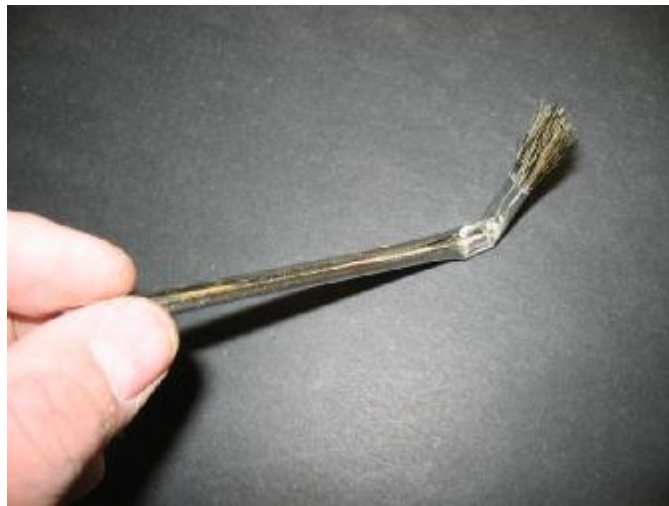
Acid brush bent for "all up and under".
