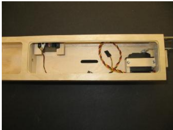
Both servos mounted. Shaft tube removed for clarity.
