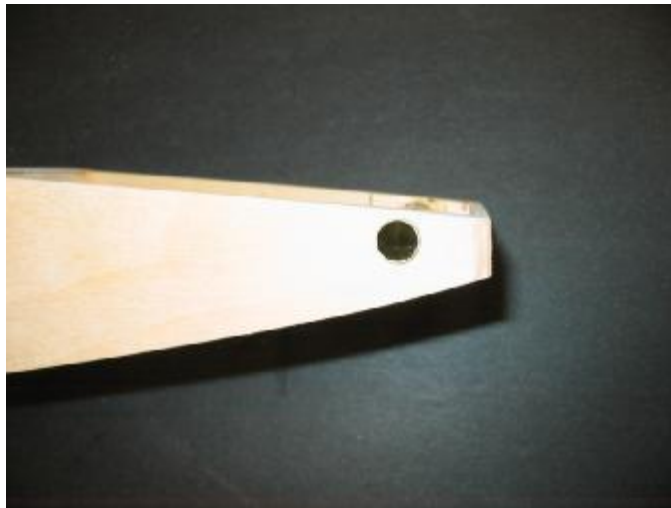
Tub sleeves sanded flush with tub side.
