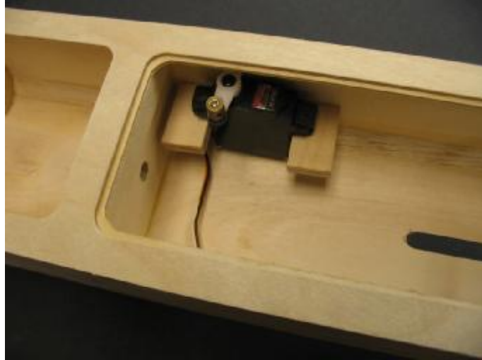
Throttle servo mounted in tub. Make sure it's on the correct side...
