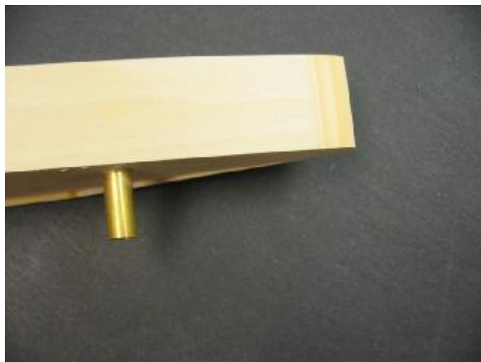
Taper side overhangs to nothing at the nose.
