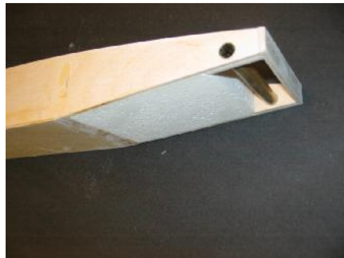
Foam sanded to match tub sides. Note angle sanded on aft sheeting.
