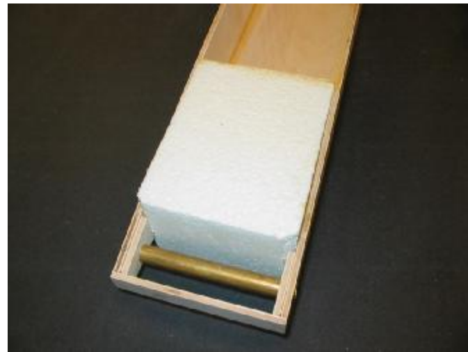
Foam nose block being test fit.
