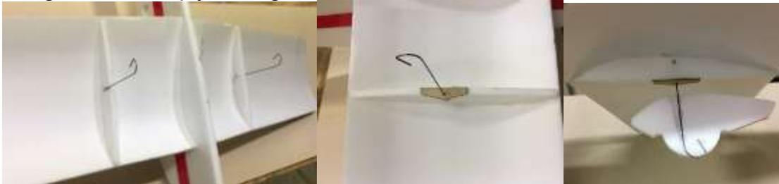
Hot glue the wheel pants in place. The mains simply glue to the outside of the wire “wheel”. Be sure to leave a tiny bit of wire “wheel” below the pant, as this will be contacting the floor, not the foam pant.
