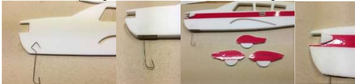
Slide the 1/32 ply nose gear brace onto the wire, and glue to fuse bottom with hot glue.
