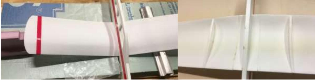
Glue each rib to the bottom of each panel about 3-1/2 inches from the fuselage. Use hot glue and hold firmly until cured. Try to get them vertical or parallel with the fuselage. Otherwise, the landing gear will be angled outward due to dihedral.
