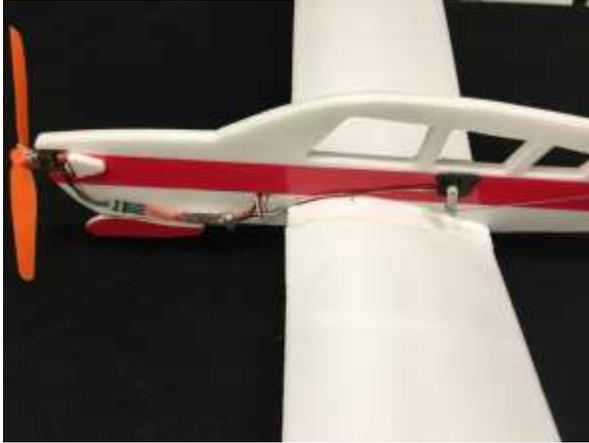
Set your battery on top of the wing, and move it around until the plane balances about 1-5/8 inches from the leading edge of the wing.
