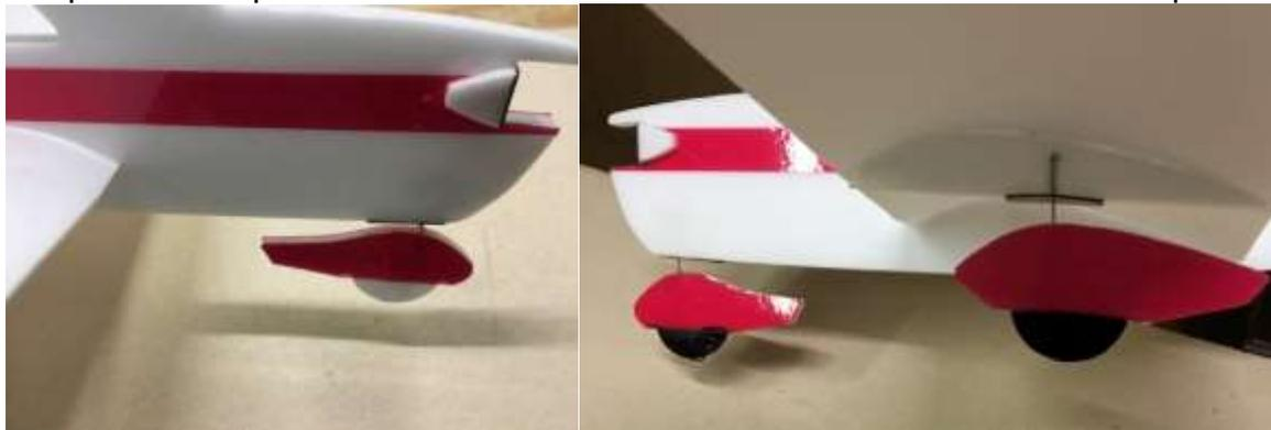
Hot glue your 3.7 gram servos into the cutout with the wires facing forward. Both servo arms should be straight down with the radio on and trims centered.
