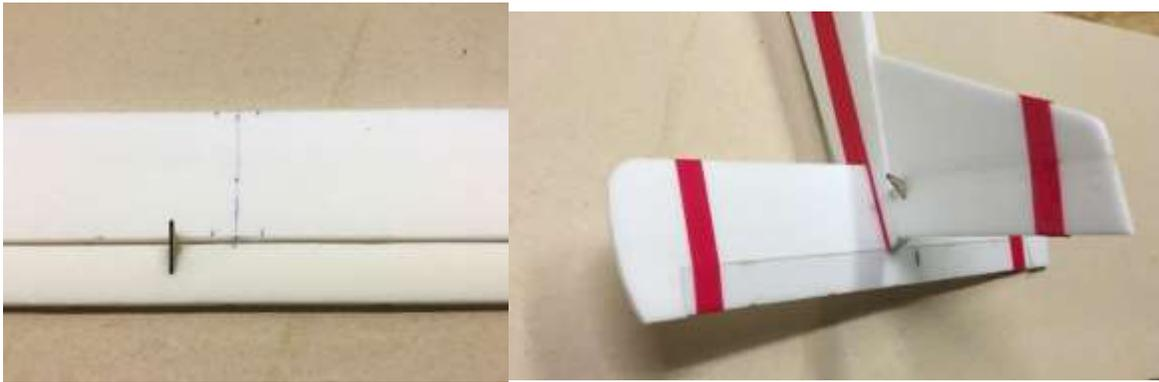
Hot glue the fin on the center of the fuse. The back of the rudder should be even with the end of the fuselage. Be sure it is straight up.
