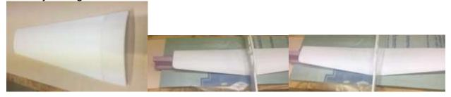
Use books or lumber to elevate the fuse, and hold it in place with the wing center section flat. You will have to allow the nose gear to hang over the table. Block up both wing tips and hot glue this panel exactly as before.
