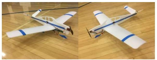
Set your battery on top of the wing, and move it around until the plane balances about 1-3/4 to 2 inches from the leading edge of the wing.
