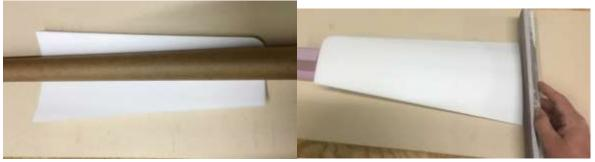
Block up the wing tip 2-3/4 inches and sand the inboard end at 90 degrees to the bench. Use a square sanding block. Put a rib under the wing, close to the end you are sanding to help hold the shape.
