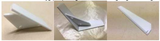
Sand or cut a bevel on the leading edge of the ruddervators.
