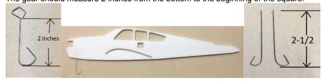
**Main gear**: Make a circle as you did before. Measure 2-1/2 inches and make a 90 degree bend about ¼ inch long. Make an opposite gear by bending the top 90 the other way. The beginning of the circle should face forward. These wires serve as the landing gear and wheels.
