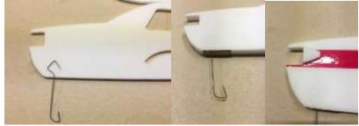
Different model shown on left. Process is the same, except the nose gear is glued 1 inch back.
