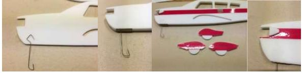
Slide the 1/32 ply nose gear brace onto the wire, and glue to fuse bottom with hot glue.
