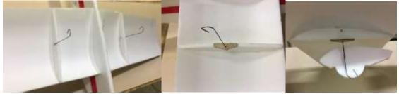
Hot glue the wheel pants in place. The mains simply glue to the outside of the wire "wheel". Be sure to leave a tiny bit of wire "wheel" wire below the pant, as this will be contacting the floor, not the foam pant.
