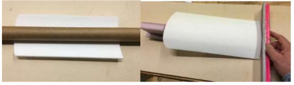
Block up the wing tip 2-3/4 inches and sand the inboard end at 90 degrees to the bench. Use a square sanding block. Put a rib under the wing, close to the end you are sanding to help hold the shape.
