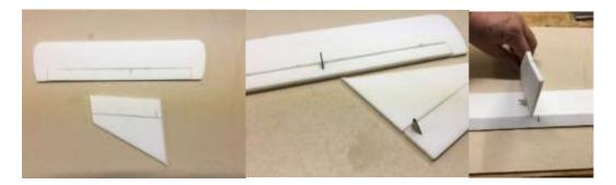
Using a tube or any round object (1-2 inches in diameter by at least 15 inches long), Roll each wing into an airfoil shape. Be sure to do a right and left (look at the wing tips). The front 1/3 has more curl than the rear 2/3.
