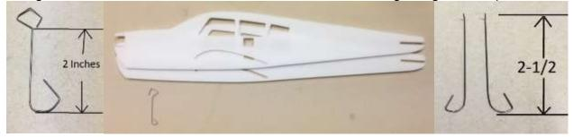
**Main gear**: Make a circle as you did before. Measure 2-1/2 inches and make a 90 degree bend about  $\frac{1}{4}$  inch long. Make an opposite gear by bending the top 90 the other way. The beginning of the circle should face forward. These wires serve as the landing gear and wheels.
