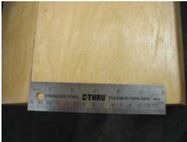
Measuring 2-1/2 inches from keel.
