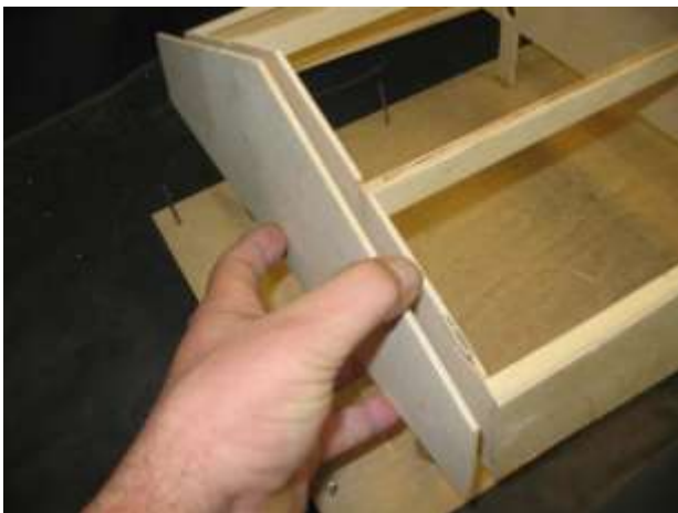
Transom being glued to bulkhead 5.
