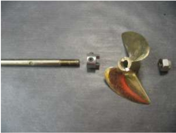
Stub shaft showing flat spot filed for set screw.
