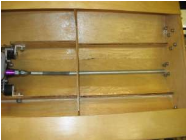
Stuffing tube aligned, ready for epoxy.
