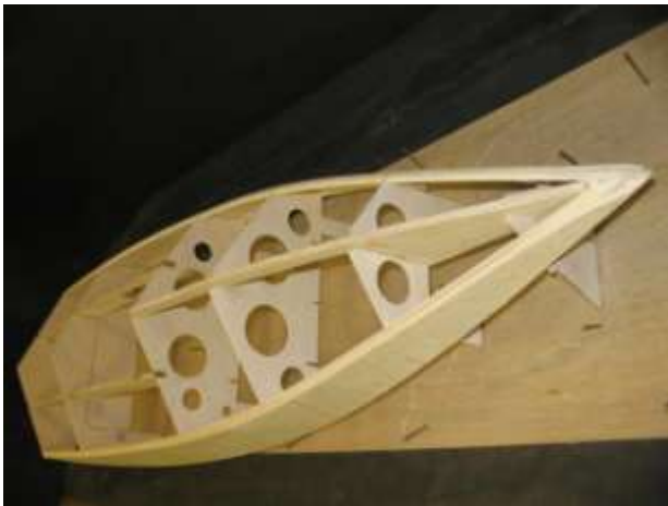
Sides and stringers planed and sanded.
