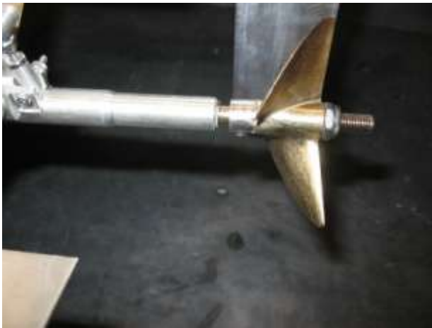
Note 1/4 inch gap at stinger drive.
