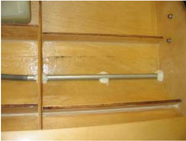
Shaft tube glued in three places.
