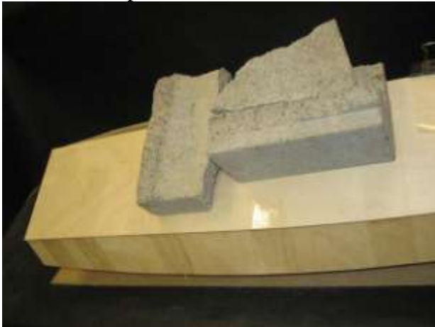
Weight applied to keep bottom sheet against engine rails.
