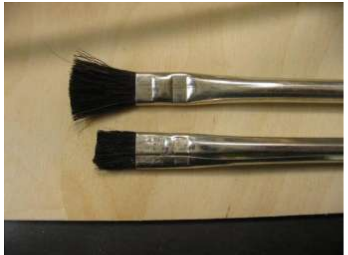
Acid brush trimmed for fast epoxy application
