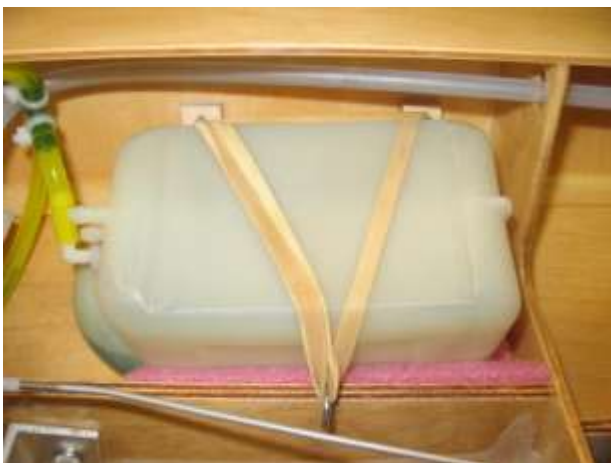
Tank held in with rubber bands. Note vibration damping foam under and beside tank.
