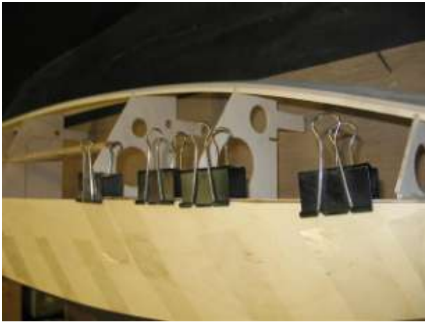
Be sure that the bottom sheet only covers half of the keel. Clamp well.
