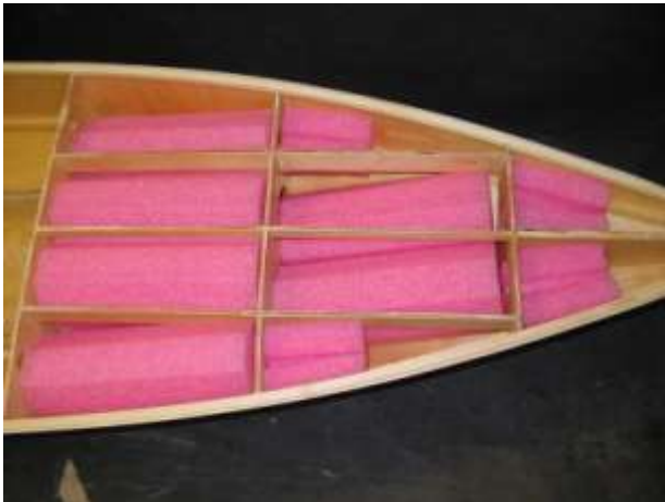
Pool noodles installed for floatation.
