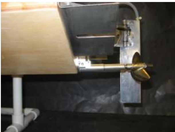
Rudder should protrude 1-1/2 to 2 inches below keel.
