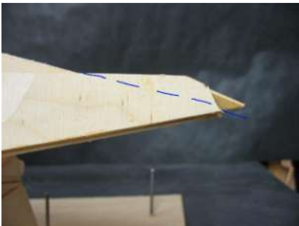
Trim sides and stringers to the same angle as the keel at the tip of the bow.
