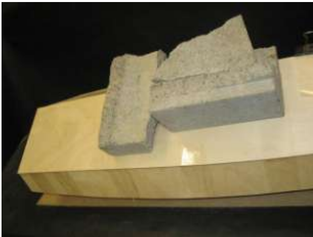
Bottom sheet taped and weighted in place.
