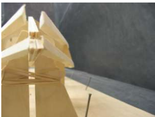
Top stringers glued flush with top of keel.
