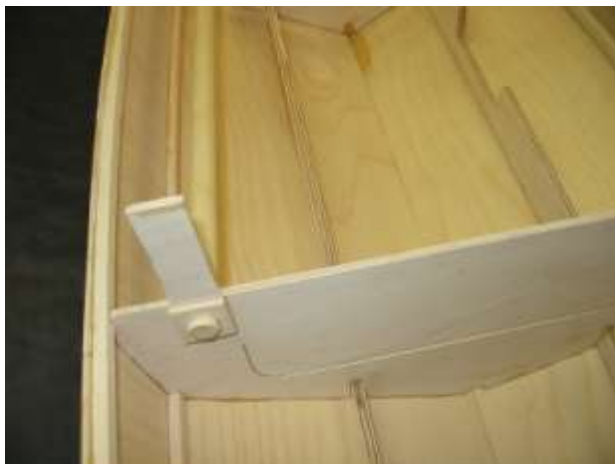
Support dowel on left side, for right handed launching.
