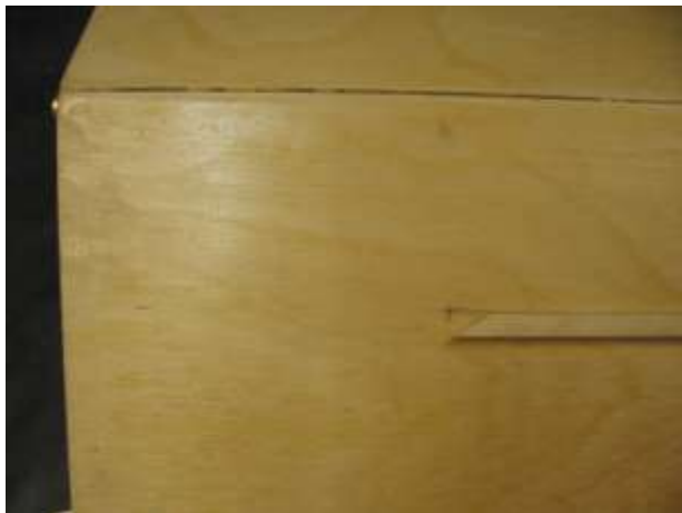
Strake in place at rear mark.
