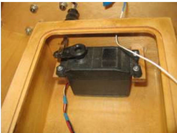
Rudder servo mounted 1/2 inch from corner.
