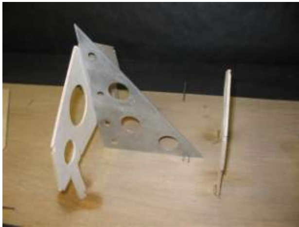
Bulkheads 1 and 2 in place.
