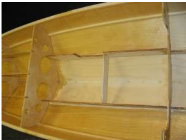
Spacer glued between engine rails maintains 5 inch spacing for engine mounts
