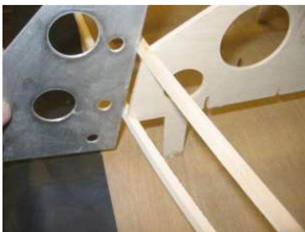
Check the stringers for flatness before gluing sides.
