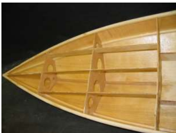
Sealing interior with epoxy finishing resin.
