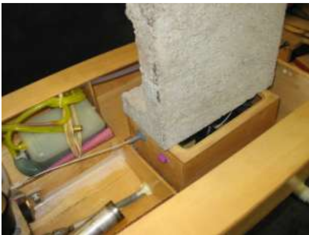
Weight holding radio box down while epoxy cures.
