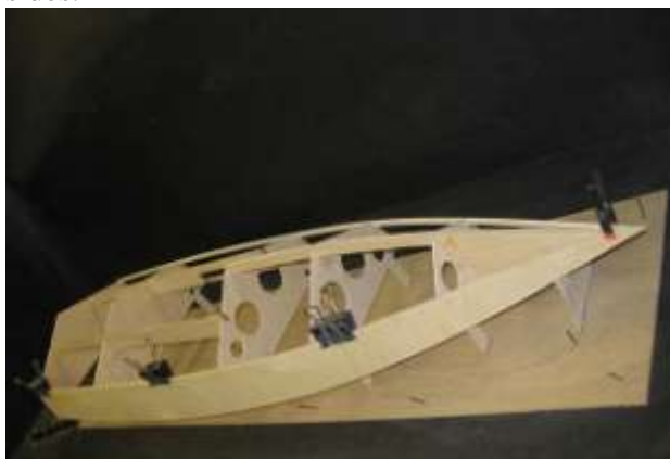
Side sheeting dry clamped in place.
