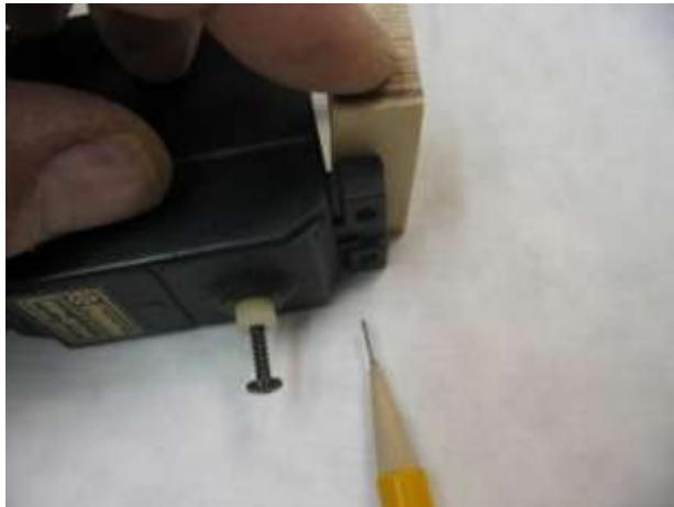
Marking servo. Be sure servo is at the end of the mount.
