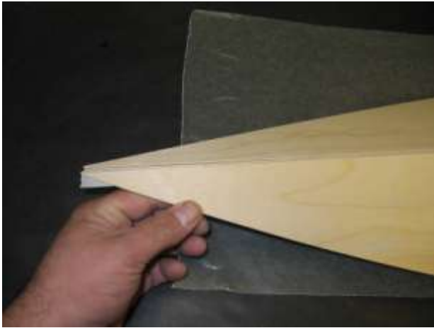
Hinging deck halves for gluing.
