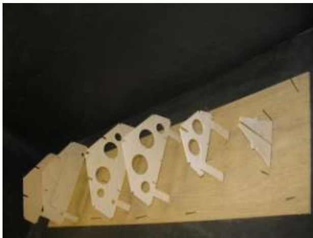
All bulkheads in place on jig..
