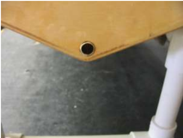
Tube cut flush with transom. Hole will be higher when using a Zenoah engine.
