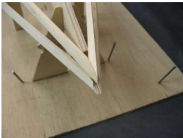
Bottom stringers glued in place.
