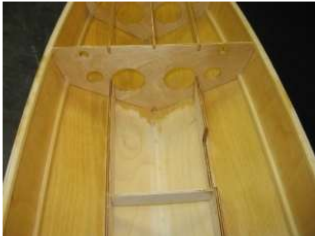
Preparing to fiberglass bottom seam. Keep spacer in place.
