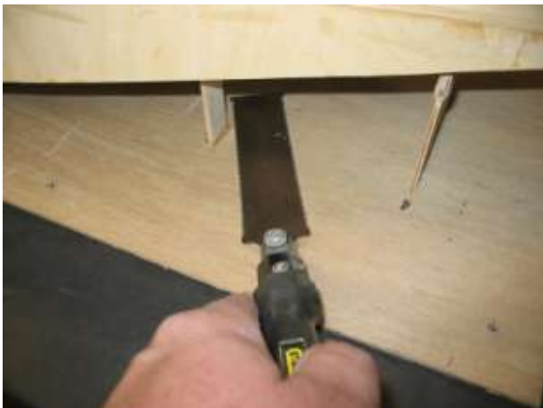
Cutting the hull free of the jig.
