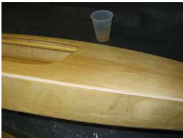
Hull sealed with epoxy resin.
