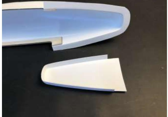
Continue to hold the chin in position and keep pushing it forward. Hold until the glue sets for a minute or two
