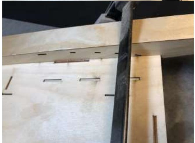
Be sure to coat the entire face of the fuselage side with epoxy.
