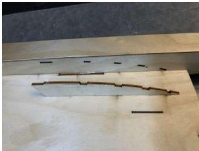
Glue the 1/16 ply (cross grain) stumble block bottom into the slots on the sponson inside, as well as into the notches on the outside piece.
