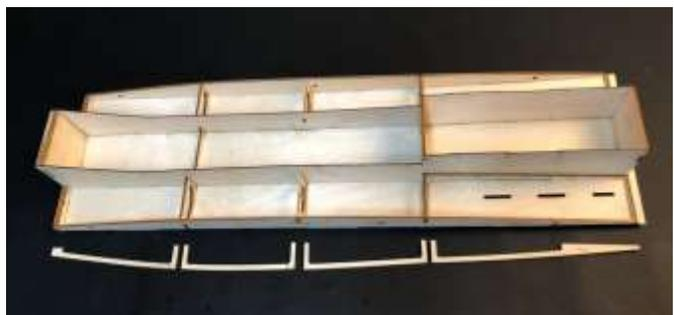
Don't glue the top decks on yet. You need two coats of sealer inside the fuselage and on the bottom of the decks.
