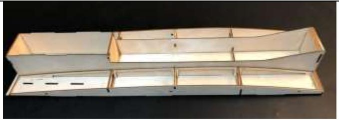
Glue the radio box lips to the bottom of the radio box top.
