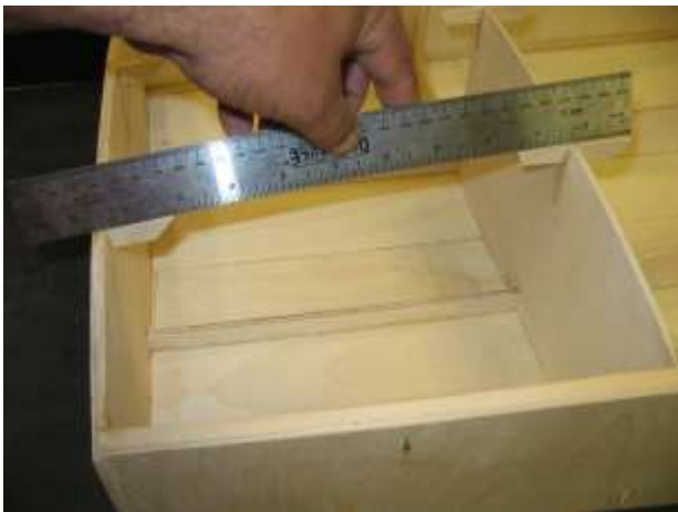
Checking deck formers with straightedge.
