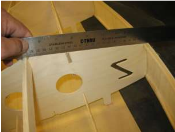
Checking the keel, bulkhead and side sheeting for flatness.
