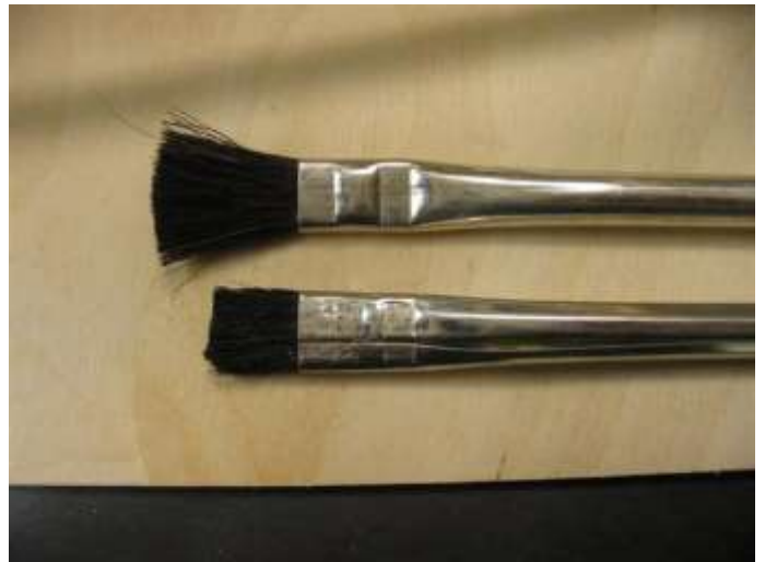
Acid brush trimmed for fast epoxy application
