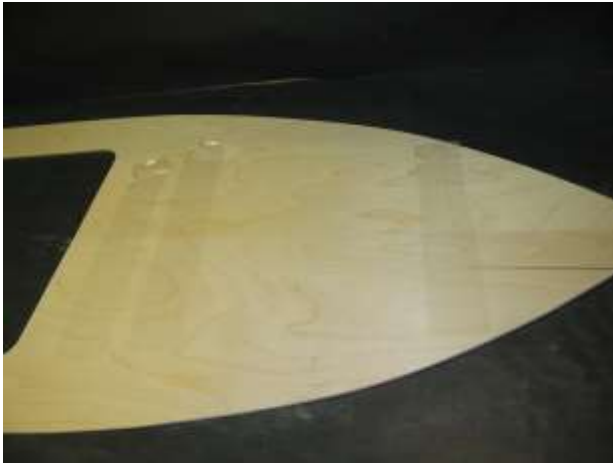
Deck pieces taped tightly together.
