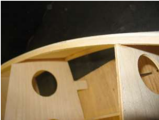
Another view of trimmed sheathing and stringers.
