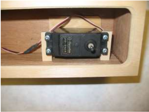
Rudder servo mounted in radio box.
