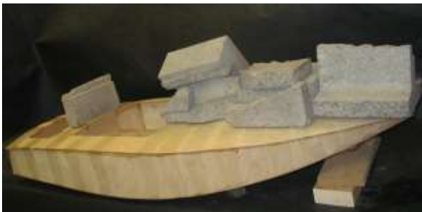
Top deck installed. Use tape and weights to get it right.
