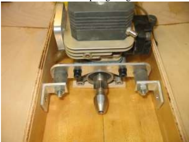
Custom mounts being installed.
