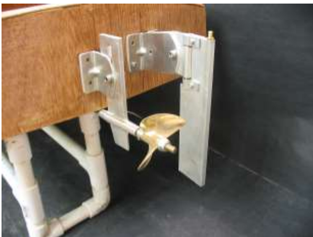
Flex shaft assembly complete.
