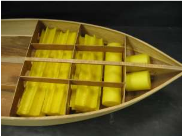
Flotation installed. Use plenty!
