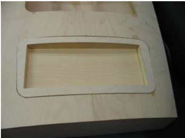
Fitting hatch to deck. Take your time here.
