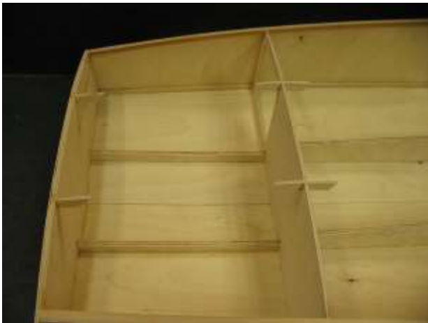
Deck formers installed in bulkheads 4 and 5.
