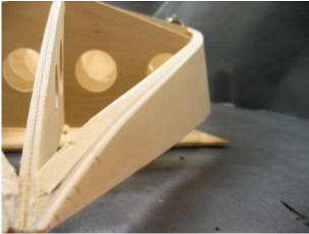
Side sheathing after trimming.
