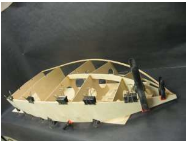
Side sheeting clamped in place.
