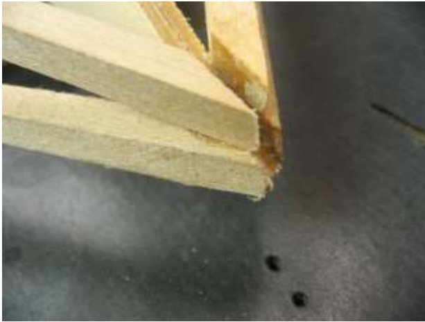
Bottom stringers glued to top stringers. Very little keel contact.
