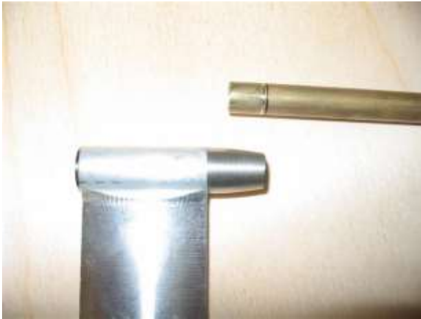
Measuring depth of shaft tube in strut.
