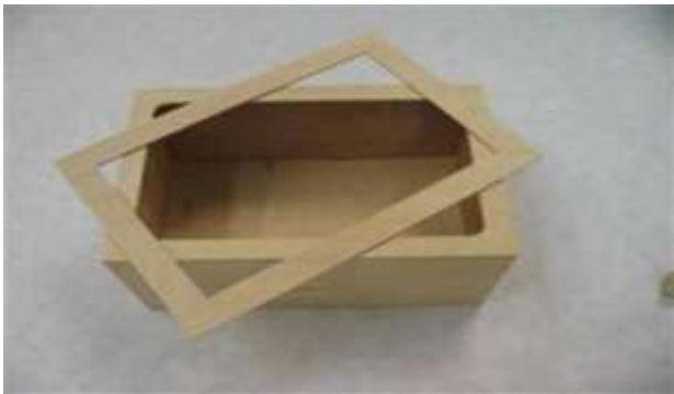
Getting ready to glue 1/8 ply top in place. Top and bottom 1/8 ply already done.
