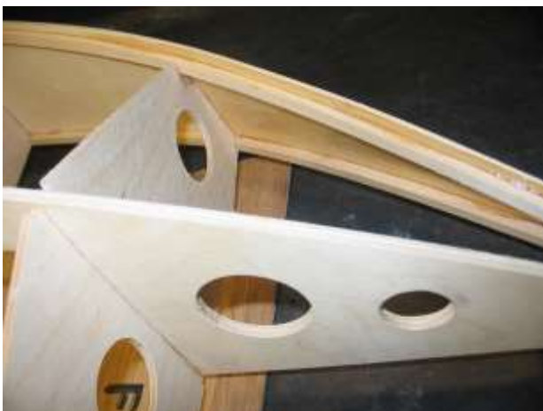
Side sheeting before trimming.
