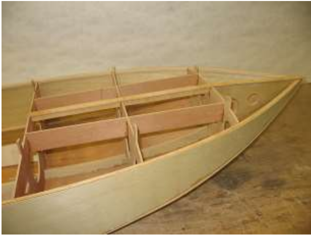
Spines and center spine installed.
