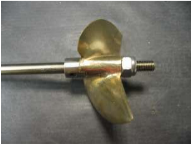
Flex shaft assembly complete.
