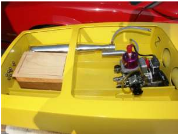
Mount the engine as far forward as possible.
