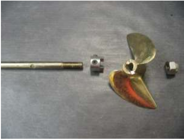
Note flat filed for drive dog screw.
