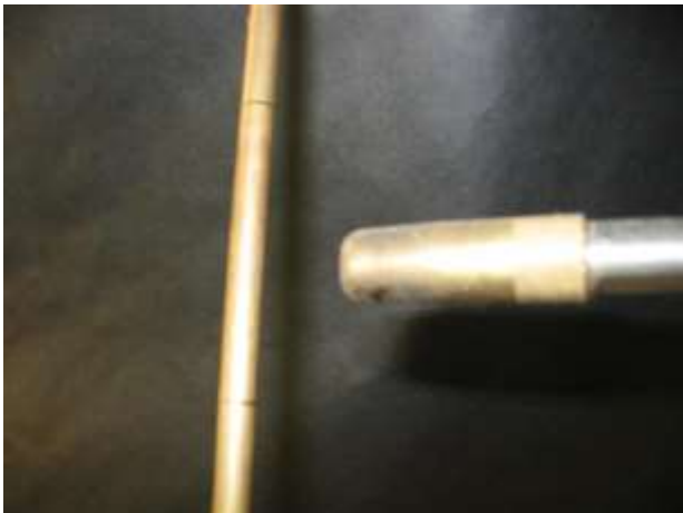
Annealing shaft tube for easier bending. Just heat until color changes.
