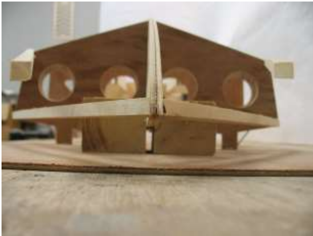
Note that top stringers are flush with top of keel.
