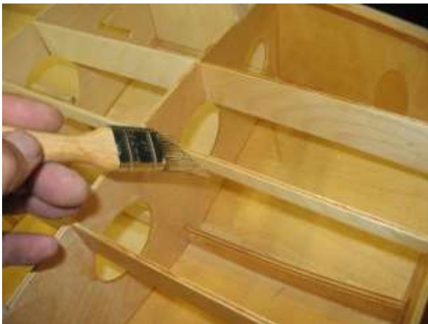
Sealing interior with epoxy finishing resin.
