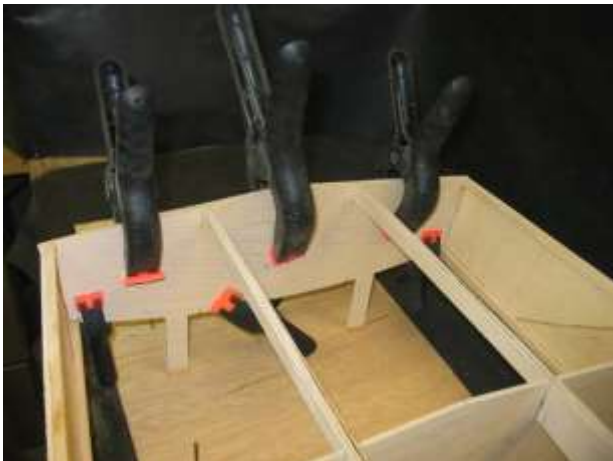
Transom glued to bulkhead 5
