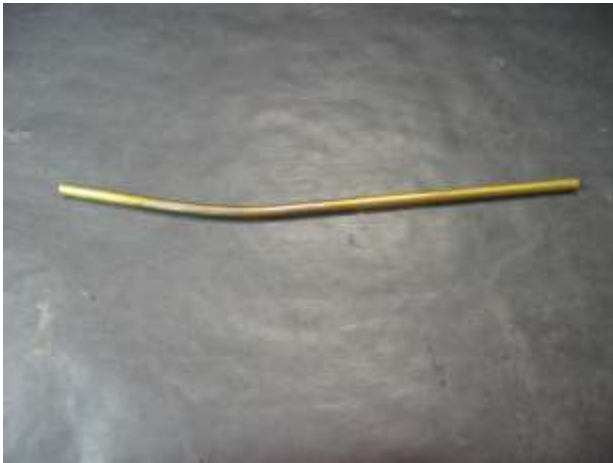
Shaft tube with smooth bend.
