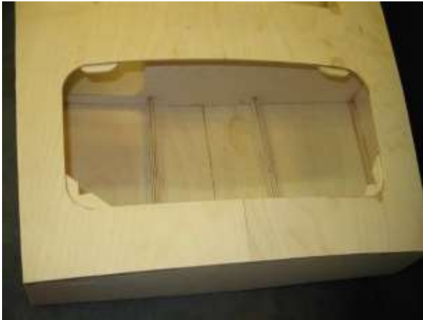
Hatch opening with tongues and bolt plates installed.
