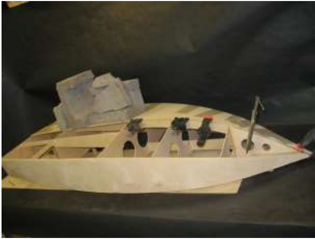
Half of bottom clamped, taped and weighted.
