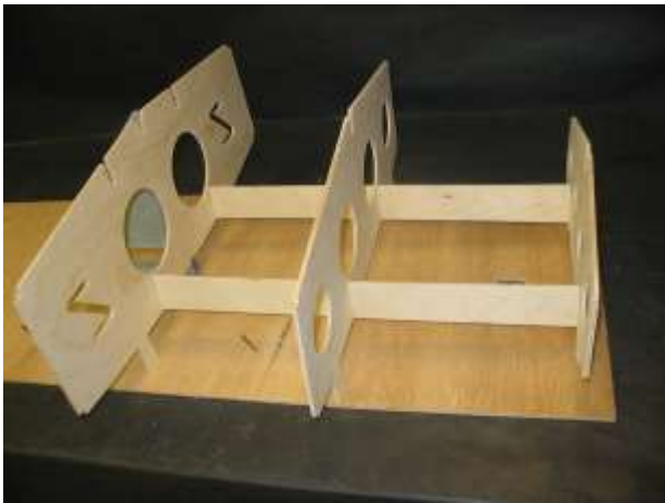
Bulkheads 1, 2 and three in place with the spines. Note that the holes in the spines face forward.
