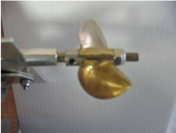
Note 1/4 inch gap between drive dog and strut.
