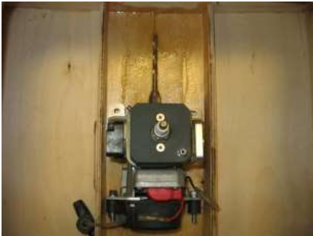
Use a 1/4 drill bit to help align engine.
