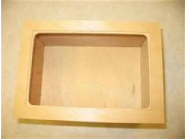
1/8 ply top installed, note lip for lid.
