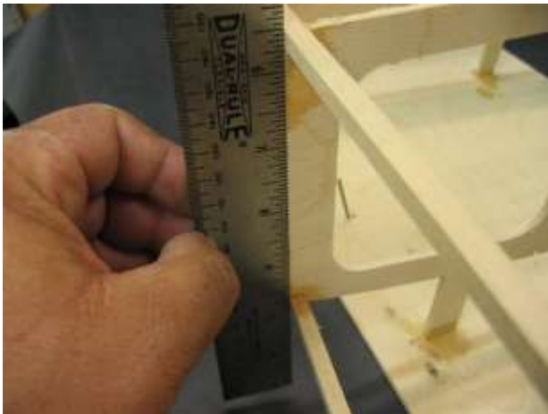
Blending stringers for a good fit of the side sheeting.
