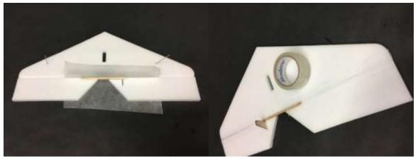
Pin the horizontal stabilizer to the bench. Use wax paper on the trailing edge and glue in the balsa elevator joiner. Don't glue the elevator to the stab. Bevel the back of the horizontal stabilizer (not the elevator). Flip the stab over and use tape for the elevator hinge. Glue the elevator ply control horn in place (the ply horn has no bevel. The rudder ply horn has a bevel).
