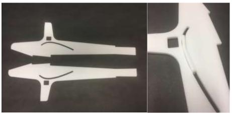
Laminate the pod doublers to each side of the fuselage. Be sure the wing slot is clear.
