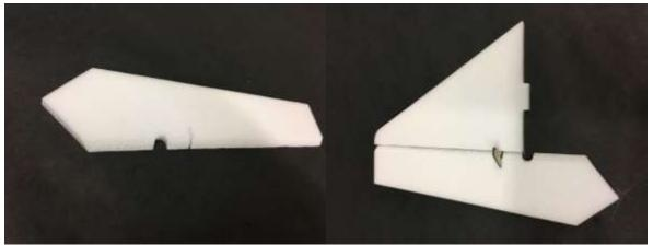
Bevel the RIGHT side of the rudder. Flip it over and tape the hinge. Flip it back over (bevel up) and glue in the ply control horn (match the bevel). Glue the fin/rudder to the stab. Make it 90 degrees. Glue the tail to the fuselage. Make it level with the wing.
