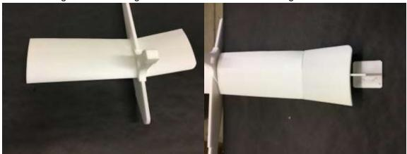
Glue the other rib in place, sand and glue the other tip in place as well. Center the wing (measure), and glue to fuse with a couple of drops of glue.
