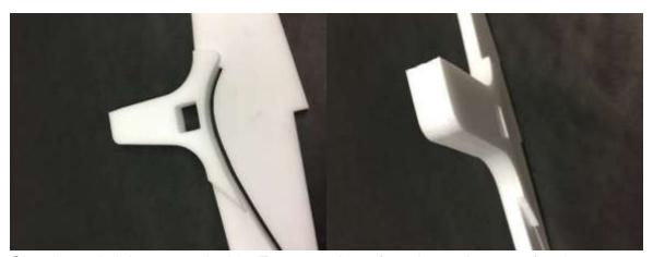
Glue the pod triplers on each side. Try to match top face, has 2 degrees of upthrust.
