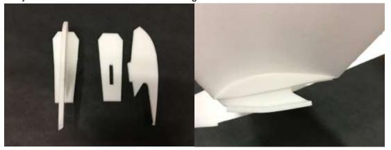
Glue the motor plate to the motor pod. You can sand the face, but try to maintain the 2 degrees of up thrust.
