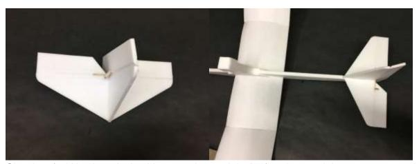
Glue the aft ski in place. It should start at the notch in the fuse bottom. It is not square, so check it against the fwd ski for orientation.
