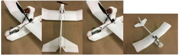
Set the battery in place, and move it around until the plane balances at 1-1/2 inches behind the wing leading edge. Use a tiny bit of Velcro to hold the battery.
