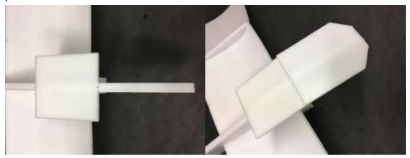
Glue the aft ski in place, as well as the fwd ski. Overlap this about 1/16 inch onto the aft ski.
