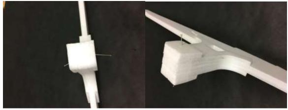
Use a pipe or tube to roll the wing and tips to an airfoil shape. Glue one of the ribs halfway on to one end of the wing center section.
