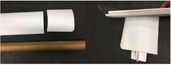
Sand the end of the wing tip slightly, so that it fits with minimal gaps when propped up on the tip dihedral gauge. Glue one tip in place, propped up.
