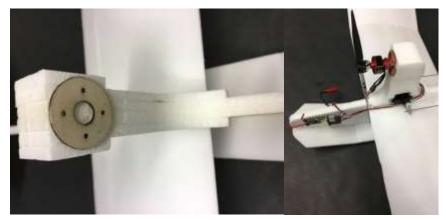
Hot glue the servos in place, as well as the esc and receiver. They should be within an inch of the nose.
