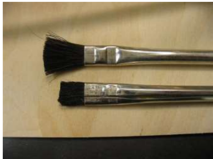
Acid brush trimmed for fast epoxy application
